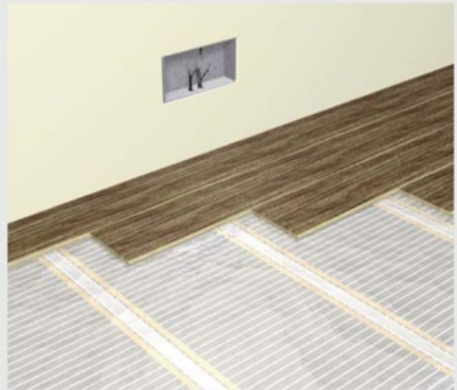
COVER ENTIRE SYSTEM WITH VAPOUR BARRIER (STOCK NO. 5415) AND LAMINATE OR ENGINEERED FLOOR IN THE NORMAL WAY
